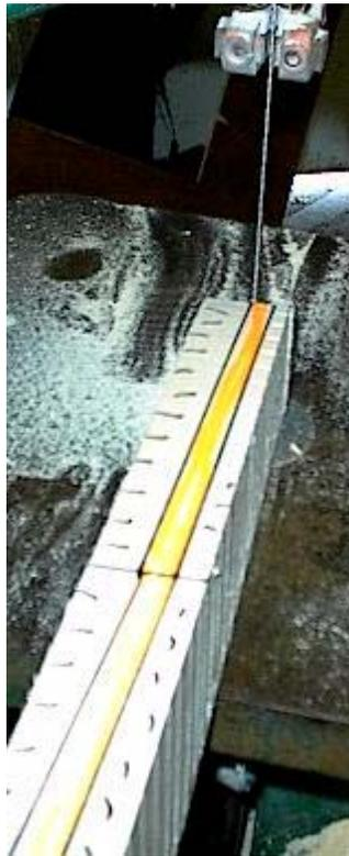
**Starting from the tip down to where it runs off the board. Be careful to cut on the outside of the line leaving a little material to work with in the end. Not critical but helpful.**
