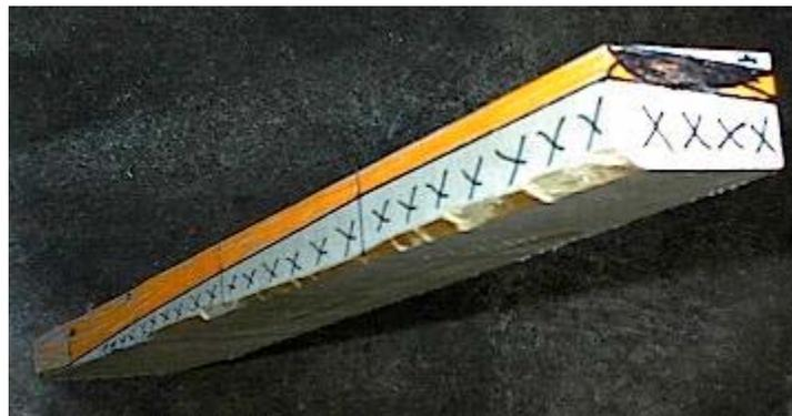
I don't like whittling little pieces for a long time to make the blade start looking like a blade so lets make some big chips fly. If you have a band saw things will go quite a bit faster but you do have to watch what you're cutting. If you don't have a band saw you can use a regular hand saw or a hack
